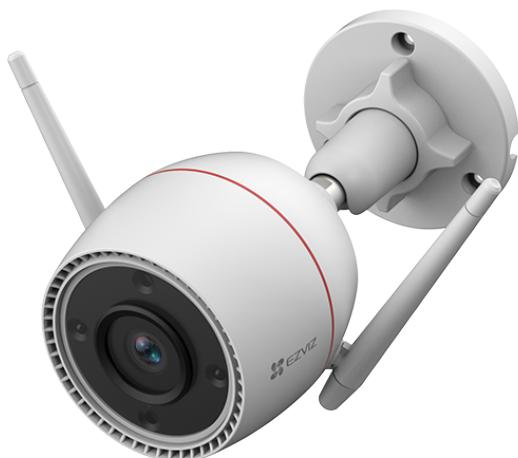
**Ezviz H3C 3MP Security Camera - 2K Resolution, AI Human Detection, Color Night Vision, Active Defence with Strobe Light, IP67, H265, Audio Pick-Up, 512GB Storage - CS-H3C-R100-1K3WKFL**
